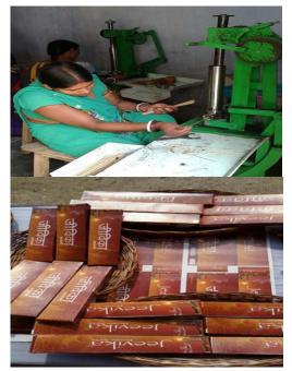
The strategy to shift from the production of hand-rolled Agarbatti to mechanized Agarbatti production is being adopted owing to the inclination of market demand towards mechanized Agarbatti. Further, this method of production is less labourintensive and time consuming. An average of 5-7 present of increase in production has been observed through the semiautomated units.
